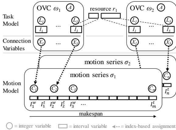
Fig. 2. Overview of CP-based STAAMS model
