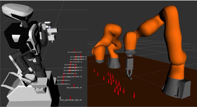
Fig. 7. A task – cleaning up the table – deployed on a KaWaDa Nextage robot (left) and a pair of KUKA LBR iiwa robots (right).
