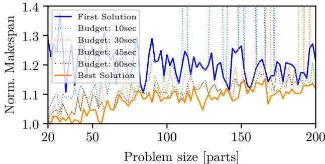
Fig. 5. In this diagram, the solution quality (makespan) divided by the lower bound (which ignores collisions between the manipulators) is shown for different problem sizes and different stages in the search. The vertical lines in the right half of the figure indicate cases in which no solution was found within the budgets of 10 or rather 30 sec.
