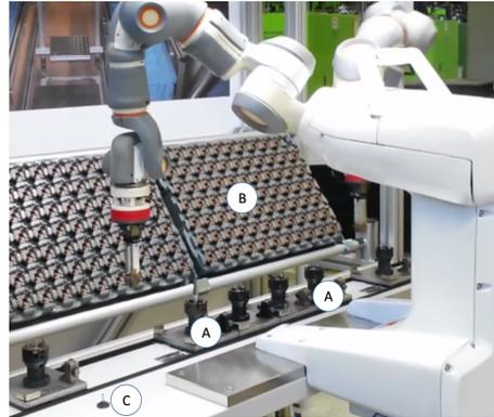
Fig. 1. Assembling of wiper motors with a dual-arm robot. The robot picks a tool from (C), places it on the shaft of the rotor of an electric motor in the workpiece holder (B), picks an electric interface, supplied in a container (B) and places it on the motor shaft.
